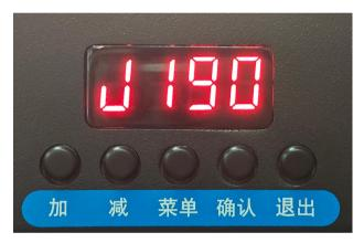
J menu MCU status, display the status code according to different configurations, no need to adjust by default
