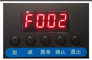
1. Press the F menu to display 1, which means that HDMI IN 1 is currently plugged in. If it displays 2, it means that it is currently HDMI IN 2.
